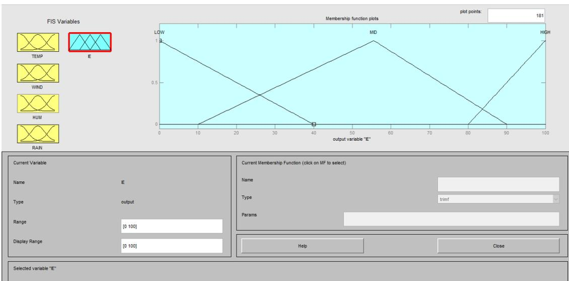
Fig 7: The membership functions for efficiency of irrigation performance output.
