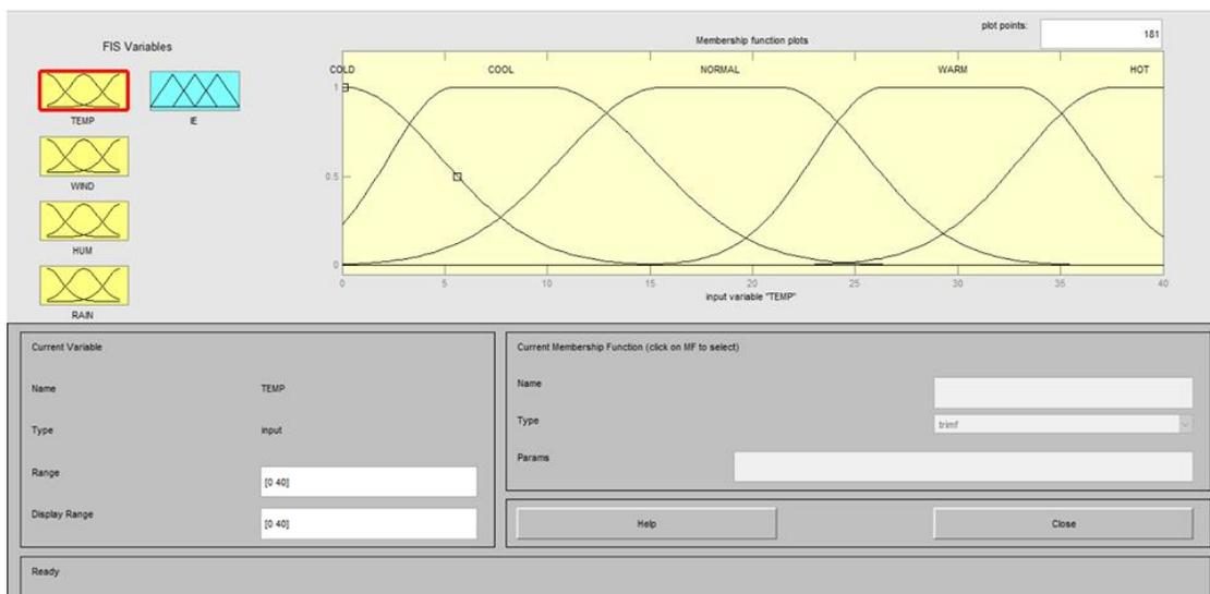
Fig 3: The membership functions for temperature input.
