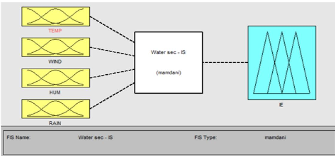
Fig 8: The Fuzzy Logic Tool Box uses simple Mamdani system
