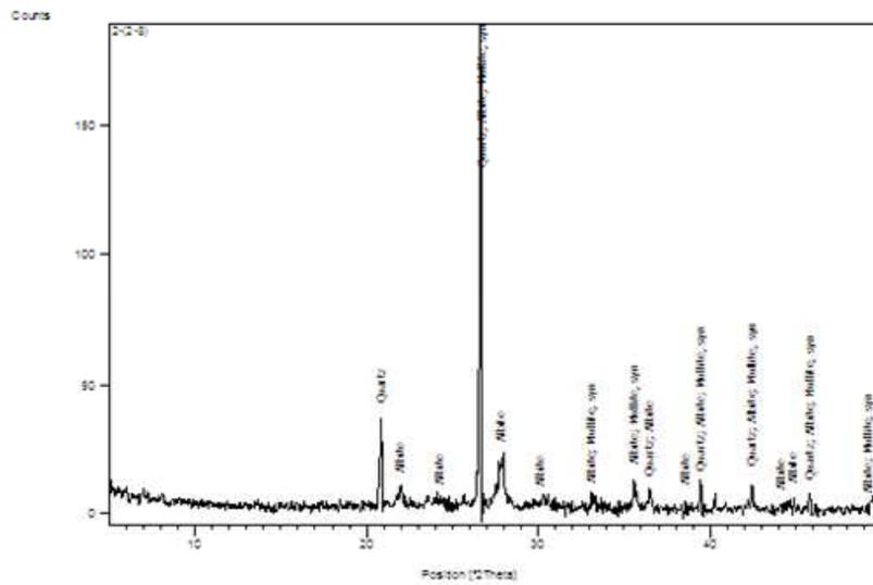
Figure 17: XRD analysis shows the mineralogical composition of the pottery disc (P<sub>2</sub>).
