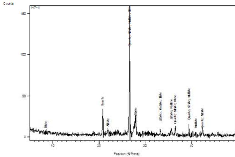
Figure 16: XRD analysis shows the mineralogical composition of the pottery disc (P<sub>1</sub>).
