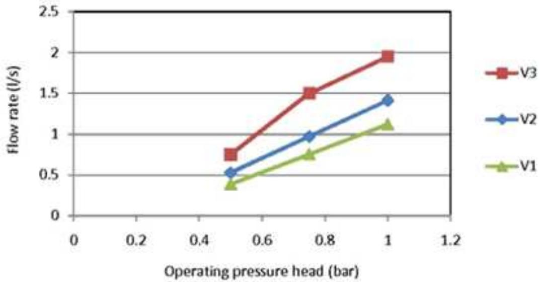
Figure 7: The effect of pressure head on pottery dripper flow rate (porosity 10 %).
