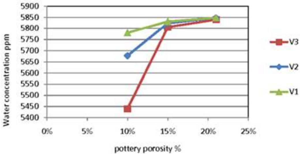
Figure 4: Effect of pottery dripper porosity of total dissolved salts (6154 ppm).
