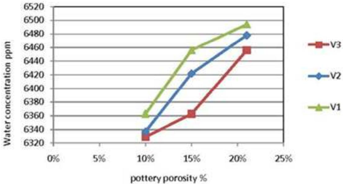
Figure 5: Effect of pottery dripper porosity of total dissolved salts (7863 ppm).
