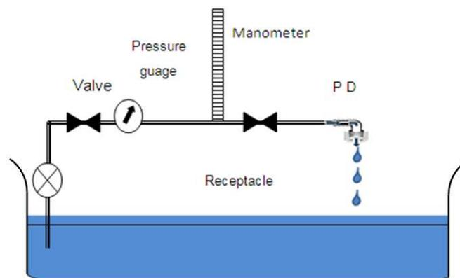
**Figure 3:** Laboratory apparatus constructed for pottery drippers (PD) experiments.
