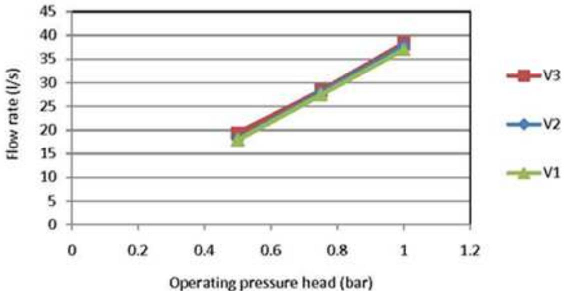
Figure 9: The effect of pressure head on pottery dripper flow rate (porosity 31 %).
