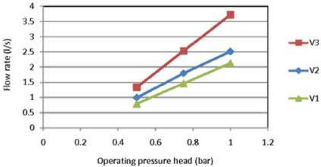
Figure 8: The effect of pressure head on pottery dripper flow rate (porosity 21 %).
