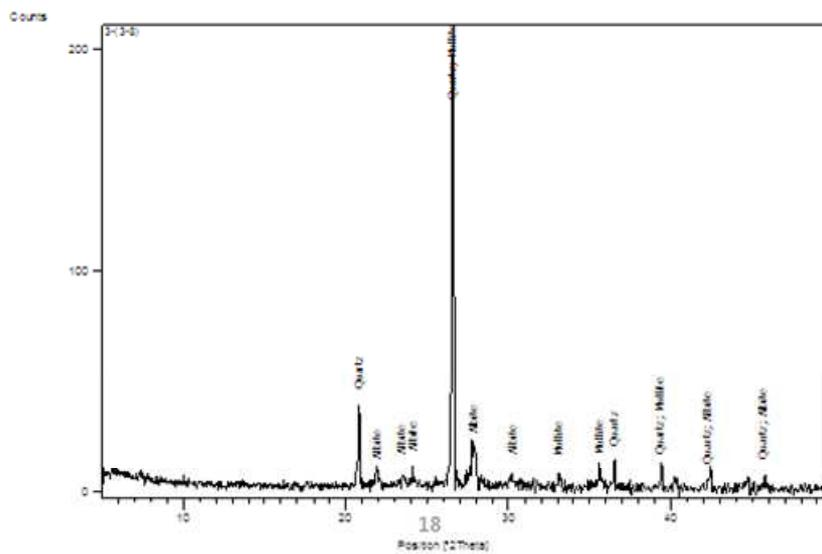
Figure 18: XRD analysis shows the mineralogical composition of the pottery disc (P<sub>3</sub>).
