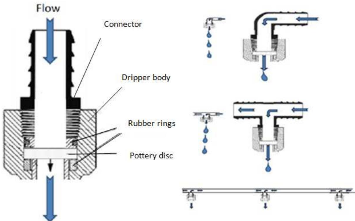
**Figure 2:** The design and proto-type of innovative pottery drippers to use the saline water in drip irrigation which under the investigation.
