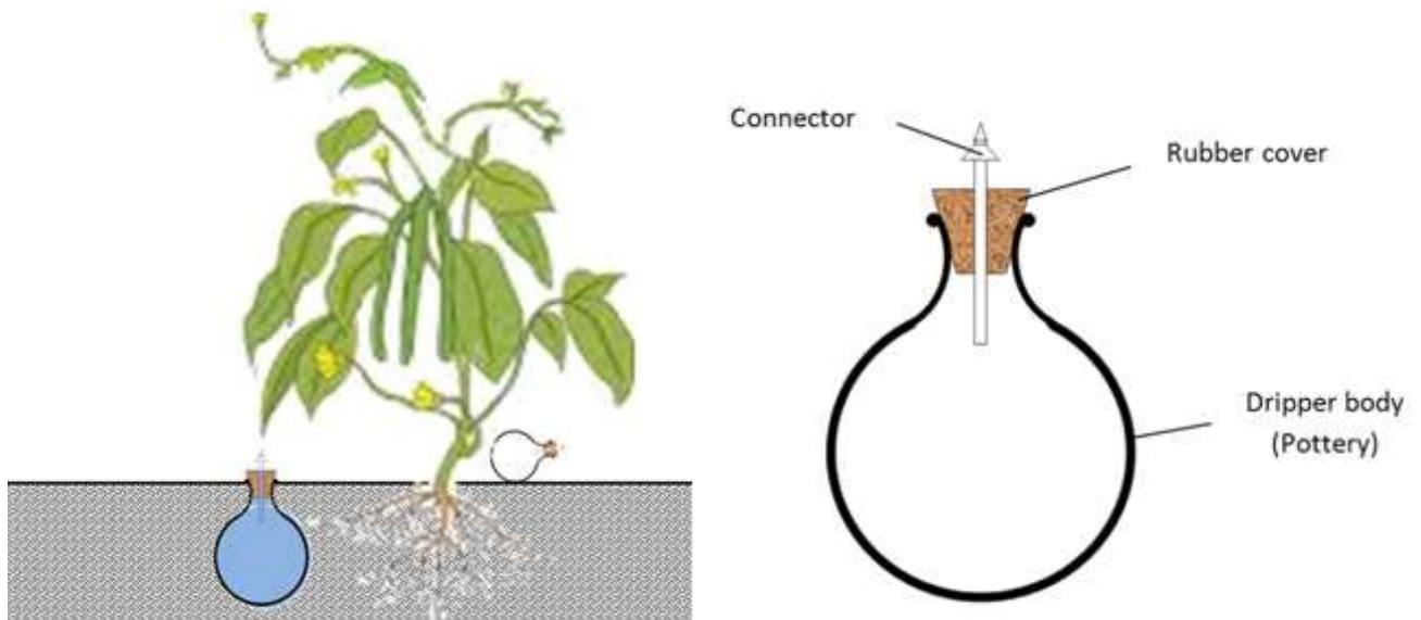
**Figure 1:** The design of pottery drippers to use the saline water in drip irrigation.
