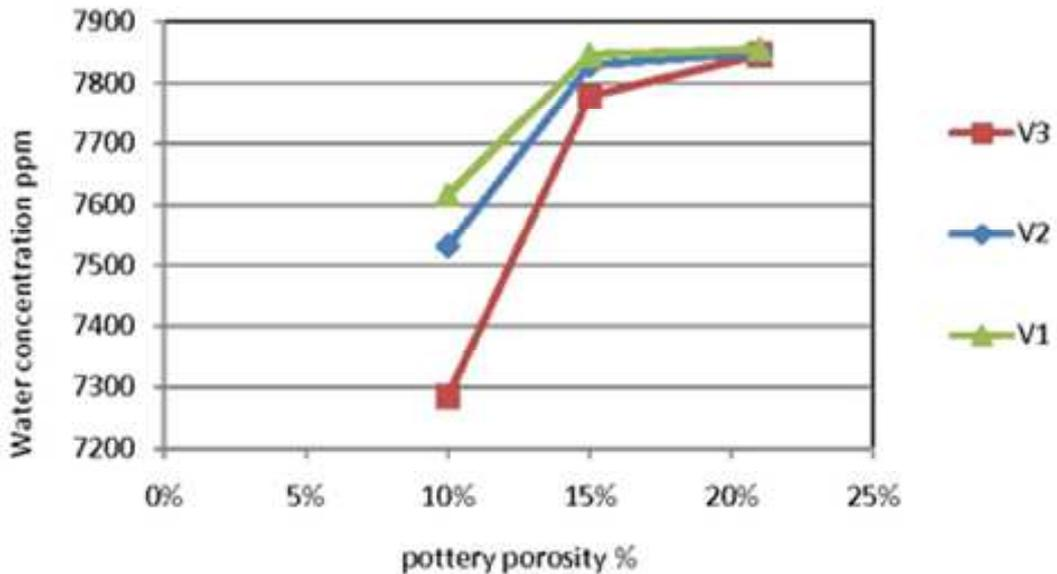
Figure 6: Effect of pottery dripper porosity of total dissolved salts (7149 ppm).
