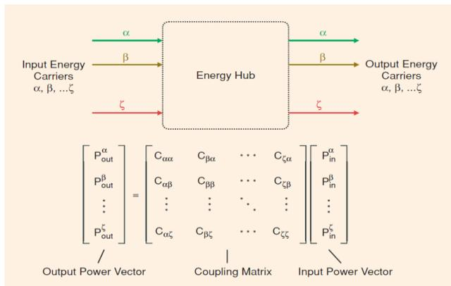
**Figure 1:** Modeling the transformation of power through an energy hub.
