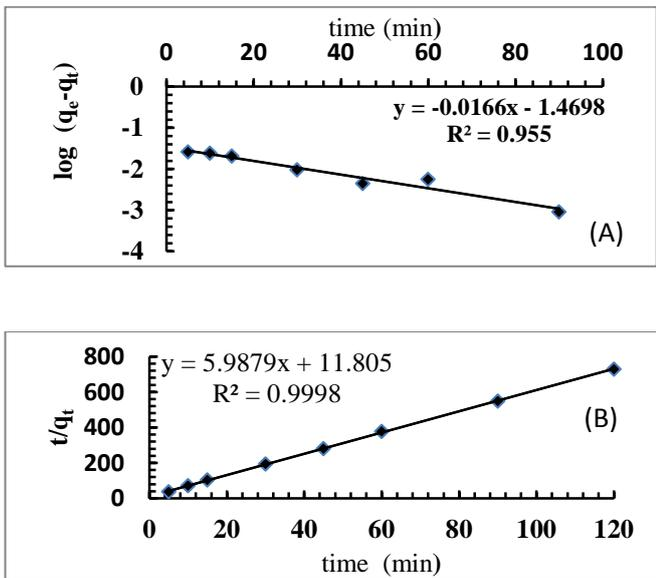
Figure (4). The adsorption of (A) pseudo second order and (B) pseudo second order Cd(II) ion from initial concentration (1 mg L<sup>-1</sup>), at 25 °C and rotation speeds 100 rpm.
