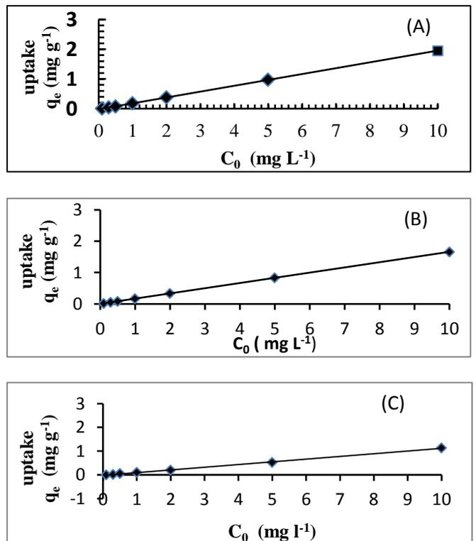
Figure (6). Effect of concentration on uptake of (A) Pb(II), (B) Cd(II) and (C) Cu(II) ions at 25 °C, t = 30, 45, 45 min and using initial pH 5, 7 and 6 for Pb(II), Cd(II) and Cu(II) ions, respectively and rotation speeds 100 rpm, using typha plant.
