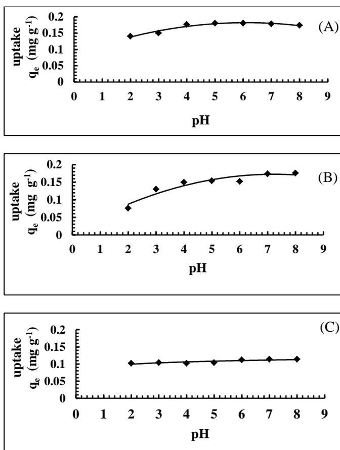
**Figure (1).** Effect of pH on the uptake of (A) Pb(II), (B) Cd(II) and (C) Cu(II) ions from initial concentration ( $1 \text{ mg L}^{-1}$ ) at  $25^\circ\text{C}$  using typha plant.
