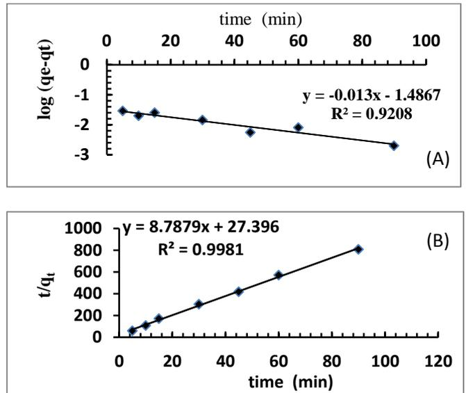
Figure (5). The adsorption of pseudo second order of The adsorption of (A) pseudo second order and (B) pseudo second order Cu(II) ion from initial concentration (1 mg L<sup>-1</sup>), at 25 °C and rotation speeds 100 rpm.
