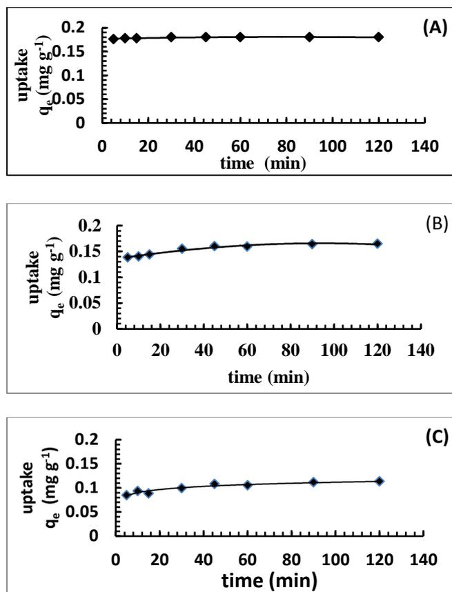
**Figure (2).** Effect of contact time on uptake of (A) Pb(II), (B) Cd(II) and (C) Cu(II) from initial concentration ( $1 \text{ mg L}^{-1}$ ) using typha plant.
