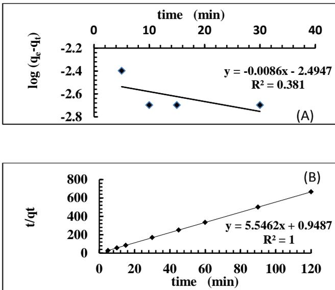
Figure (3). The adsorption of (A) pseudo second order and (B) pseudo second order Pb(II) ion from initial concentration (1 mg L<sup>-1</sup>), at 25 °C and rotation speeds 100 rpm.
