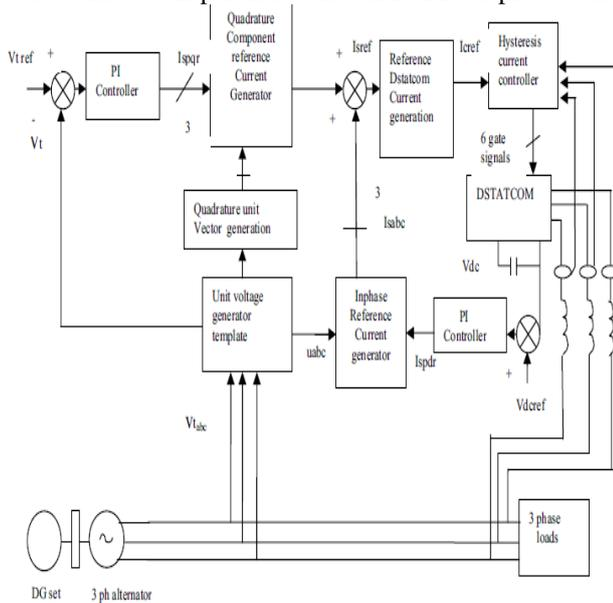
**Figure 3:** Control scheme of D-STATCOM for Isolated Alternator System driven by Diesel Engine
