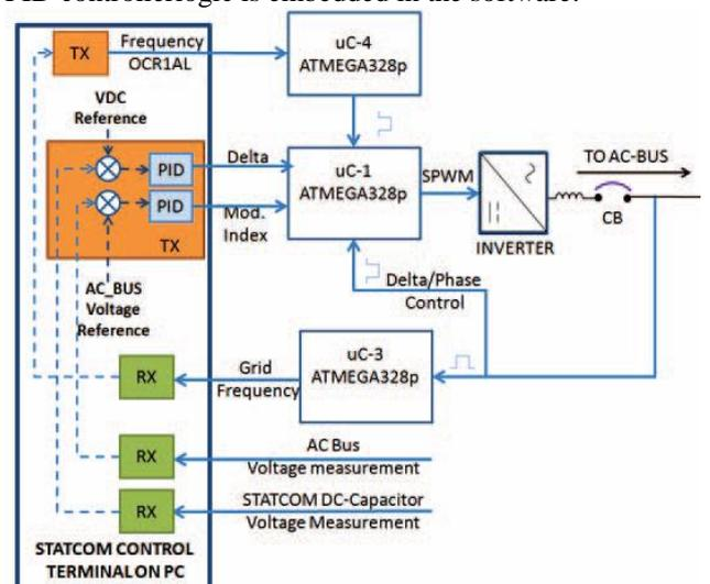
**Figure 2:** STATCOM control system schematic
