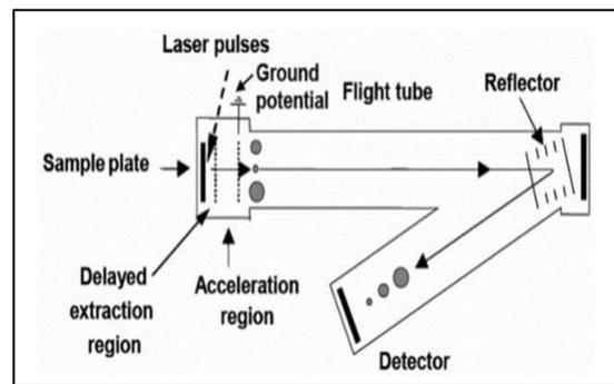
**Figure 2:** Schematic illustration of a MALDI-TOF/MS
