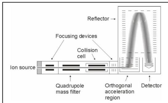
**Figure 1:** Schematic illustration of the principal components of ESI-MS
