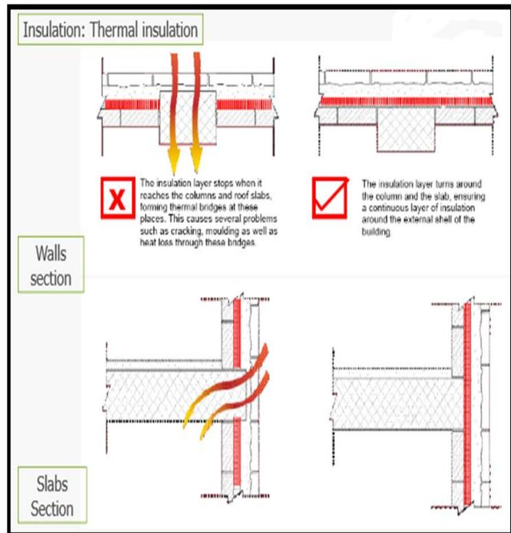
**Figure(7):** The thermal isolation in Passive Design
