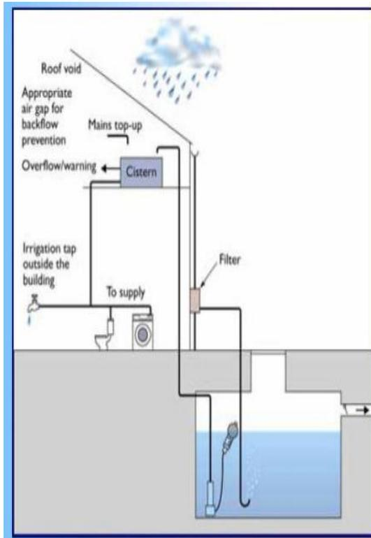
**Figure(3)** : A schematic of an indirectly pumped system
