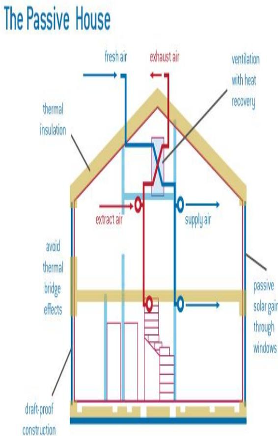
**Figure(5):** The general design system in Passive Design
