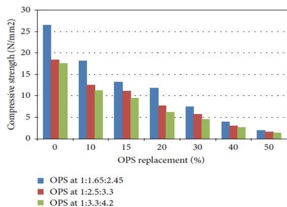
**Figure (3):** A comparison of compressive strength of OPS at 7 days of curing
