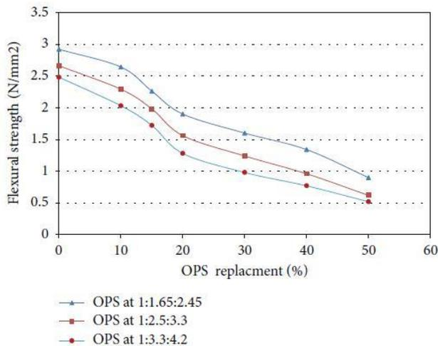
Figure (4): Comparison of flexural strength of OPS at 7 days of curing
