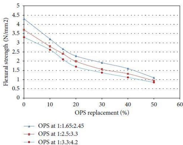
Figure (5): Comparison of flexural strength of OPS at 28 Days of curing
