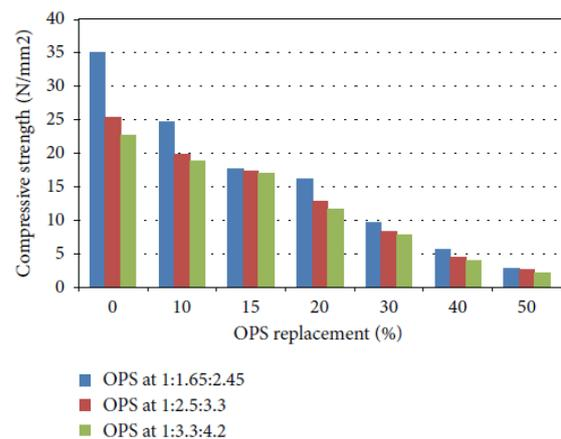
**Figure (2):** A comparison of compressive strength of OPS at 28 days of curing
