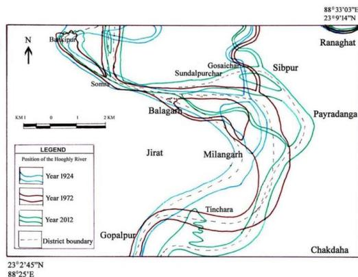
**Fig 3:** Position of the Hooghly River channel
