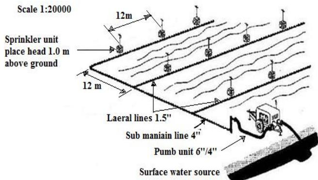
**Figure 1: Layout of the fixed sprinkler irrigation system.**
