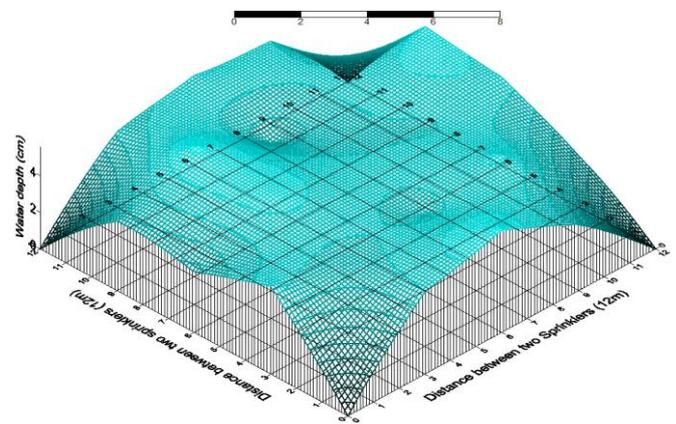
**Figure 4: Three dimension model of the water distribution by permanent sprinkler irrigation system.**
