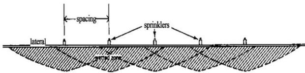
**Figure 3: Soil wetted zone within overlapping under the fixed sprinkler irrigation system**
