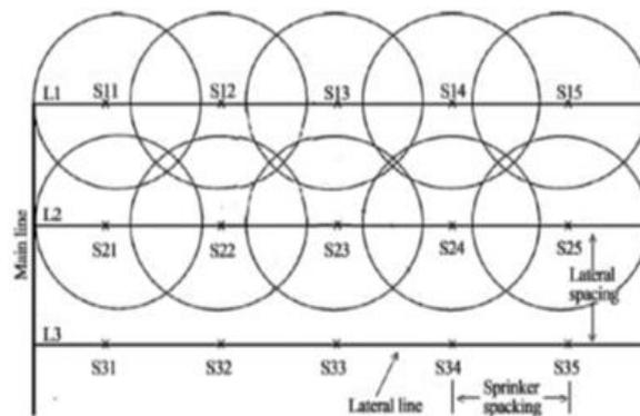
**Figure 2: Lay out of the fixed sprinkler irrigation system with detail components and sprinklers overlapping.**
