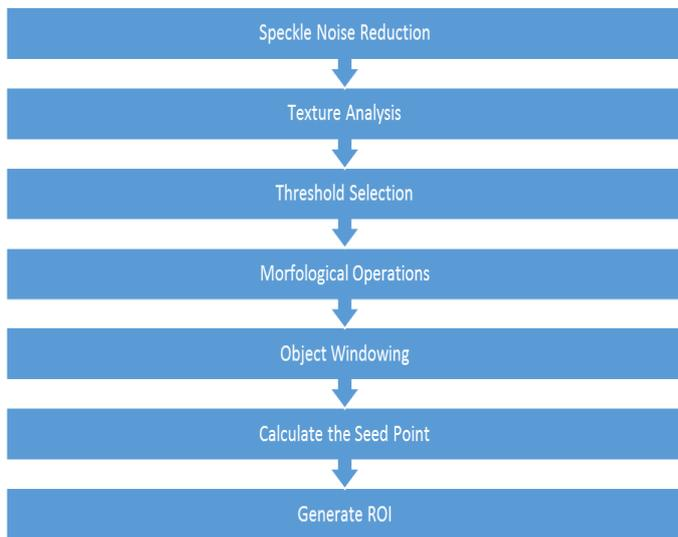
Figure 4: Block Diagram of ROI Generation
