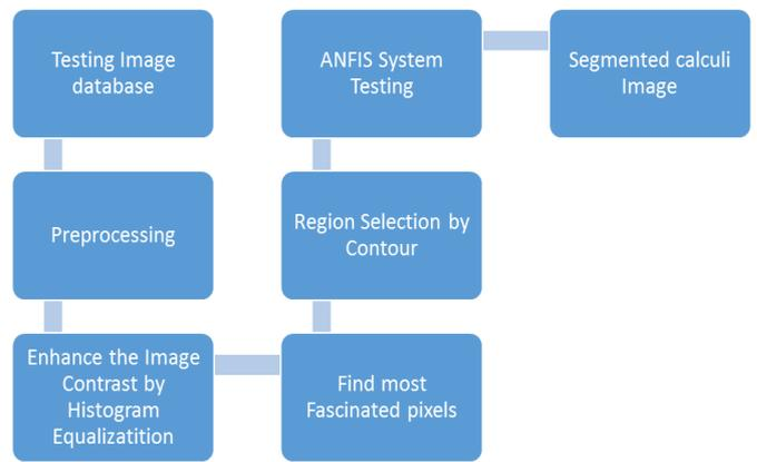
Figure 3: KSST Segmentation Method
