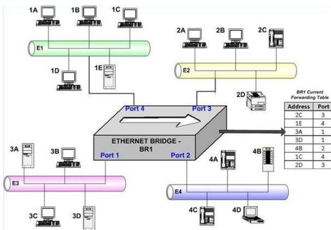
Fig - 1 : 4 Port Bridged Ethernet joining Ethernet Segments E1, E2, E3, E4
