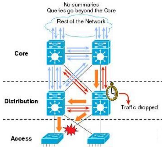
Fig-3 : Model for controlling bandwidth during traffic within the network
