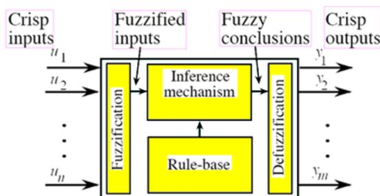
**Figure 3:** Basic parts of a Fuzzy Controller
