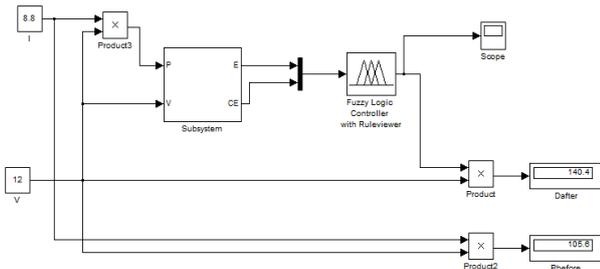
Figure 17: Output of the solar system using FLC
