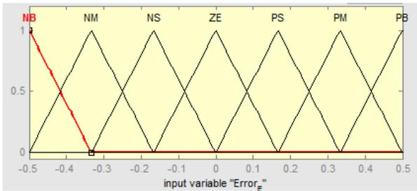
Figure 6: Input Membership function for given error
