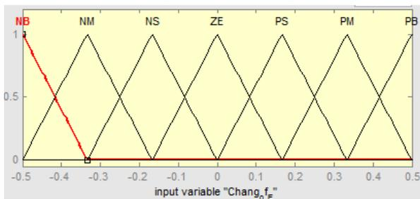
Figure 7: Input Membership function for change in error
