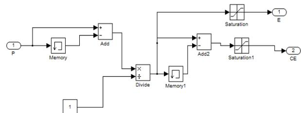
Figure 15: Generating the Error and Change in Error
