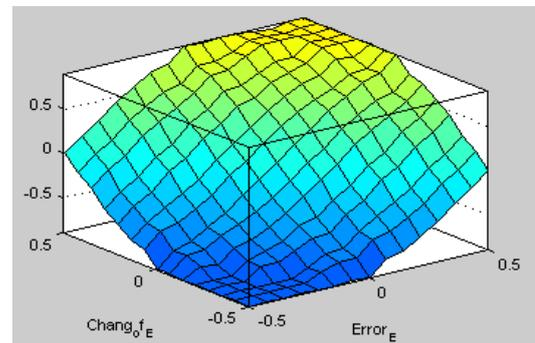
Figure 10: Surface shape (E, ΔE and output I)
