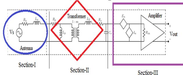
**Figure.2:** System design of fully differential magnetic field receiver, including antenna model, transformer model, and noise model of amplifier
