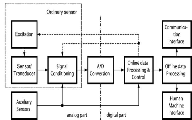
**Figure 1:** The structure of an intelligent sensor.
