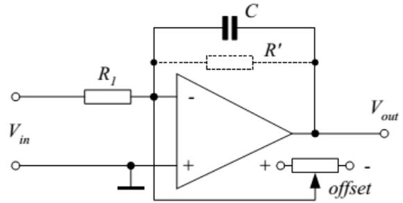
**Figure.4:** The integrating circuit for the coil
