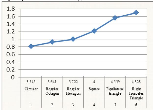
Graph gain between types of loop Inductive coil sensor
