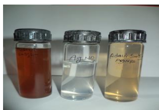
Figure 3: Ocimum basilicum L. var.thyrsoiflorum leaf extract, aqueous AgNO 3 , Silver nano particles and color change respectively.
