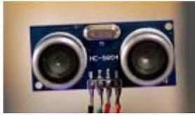
**Figure 1:** Ultrasonic Smart sensor
