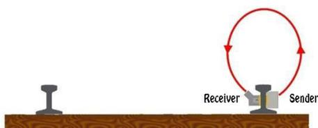
Figure 6: How to count the number of axle by axle
