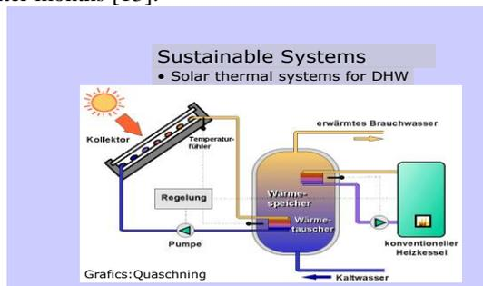
**Figure 5** Proposed heating warm water system thru solar energy
