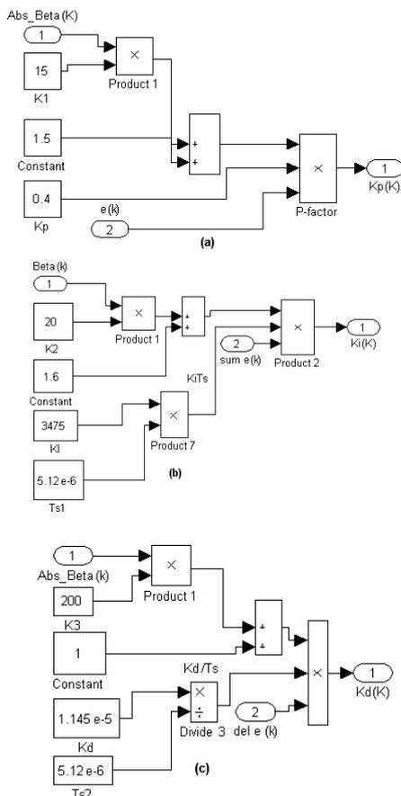
Figure 11 : Modified controller gains (a) Proportional (b) Integral and (c) Derivative
