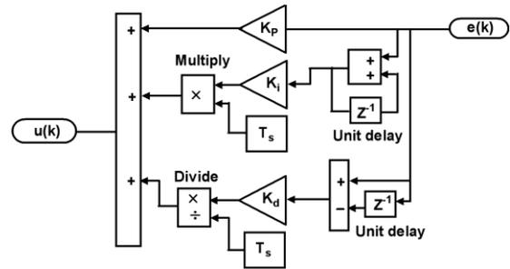
**Figure 7:** Discrete form PID Controller structure
