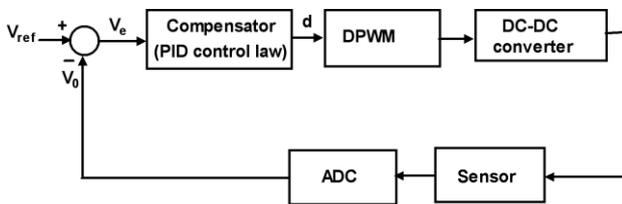
**Figure 6:** General PID-based feedback Control of switching converter
