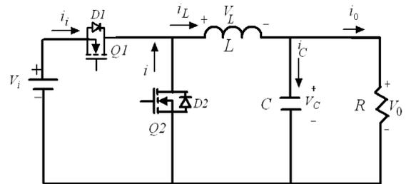
Figure1: Power stage of synchronous buck converter
