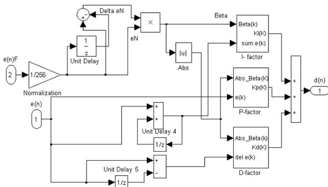
Figure10: Simulink model of Fine-tuned PID Controller structure for DC-DC Converter
