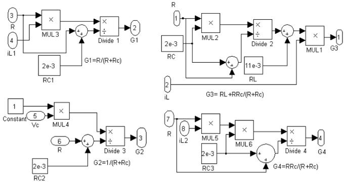
Figure 4: Simulink model of sub-systems G1, G2, G3, and G4 of Figure 3
