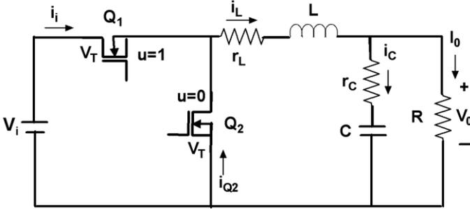
Figure 2: Buck converter with non-ideal components
