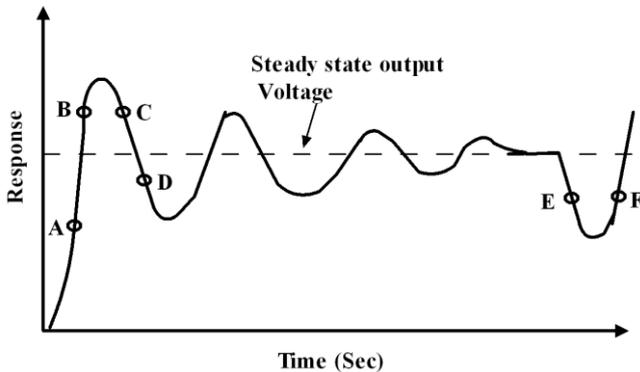
**Figure 9:** Typical closed loop response of DC-DC converter as second order (Under damped) system
