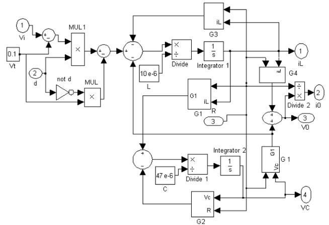
Figure 3: Simulink Model of buck converter (Power stage)
