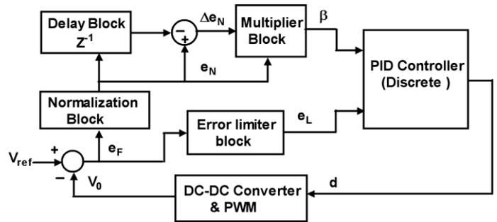
**Figure 8:** Block diagram of Fine-Tuned Discrete PID Controller structure
