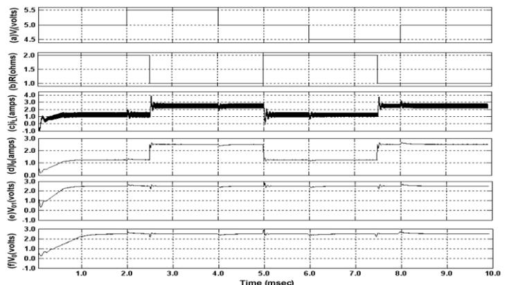
Figure13: Closed loop response of buck converter-(a) Input source voltage  $V_i$  (b) variation in load resistance  $R$  (c) Inductor Current ( $i_L$ ) (d) load current  $i_0$  (e) output voltage of converter with normal PID Controller (f) output voltage of converter with Fine-tuned Discrete PID Controller
